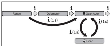
By pressing the “i” button for more than 1 s, you can switch back and forth between the “**Gear: Auto**” automatic mode and the “**Gear**” manual mode.
