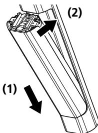
**2.1.6 Removing an integrated type battery****1. If there is a separate plastic cover for the battery in place, remove this from the bicycle first.****2. Release the battery lock.**
