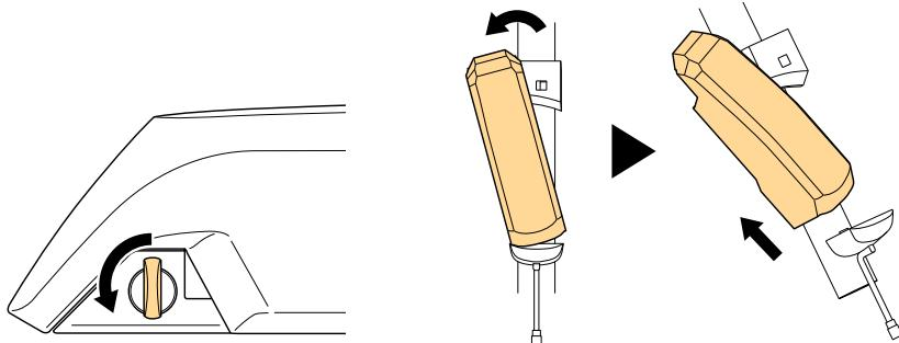
**2.1.5 Installing an integrated type battery****1. Use the following procedure to insert the battery from the bottom.**
